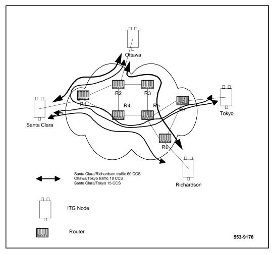
To complete this exercise, total the traffic flow from every site pair to calculate the load on each routed and loaded to the link.
